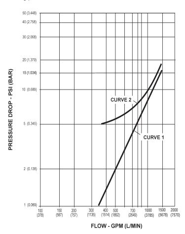
Curve 1 Pressure loss of Model 61525 mated with Model 60505 Adapter Pressure loss of Model 61525 mated with Model 60554D Hydrant Valve
