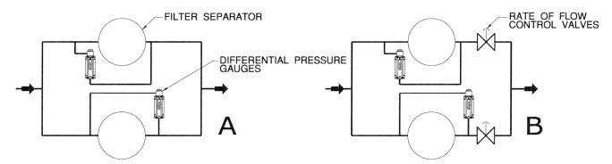
Now that we have covered the necessity of limiting the flow rate, we must remind you that a differential pressure reading means very little unless you know the flow rate. This was covered in GamGram 26.
